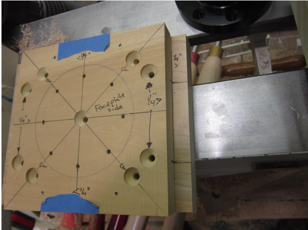
Picture 12 – The mounting holes for the first offset have been drilled, and the faceplate board holes enlarged so the screws can pass through.
