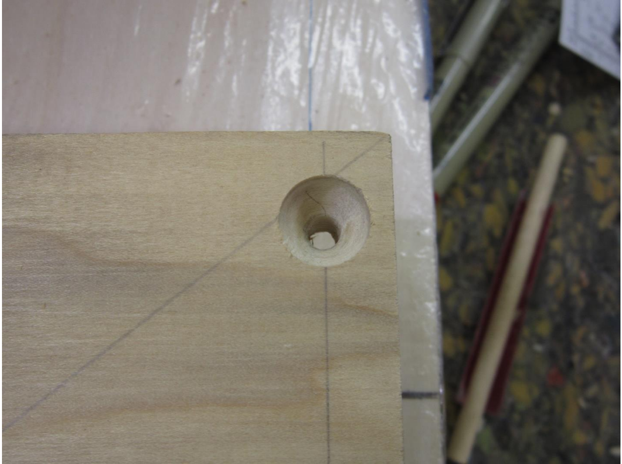
Picture 01a – countersunk screw hole (detail). Note the tapered hole to support the head of a typical wood screw.
