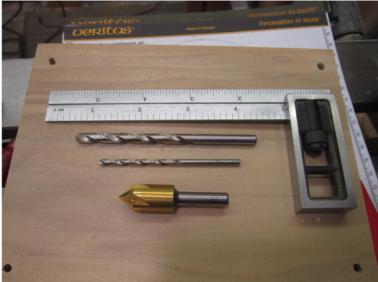
Picture 01 – Tools used. From top to bottom: square, large drill bit (approx 1/4" dia.), small drill bit (approx. 1/8" dia.), 60 degree countersink bit.
