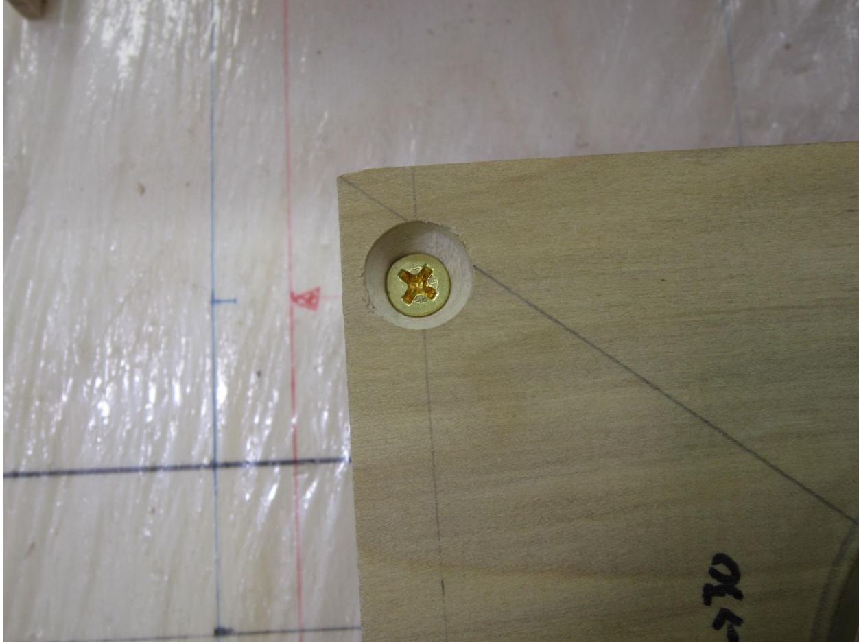
Picture 01b – Brass wood screw seated in and supported securely by the countersunk screw hole.
