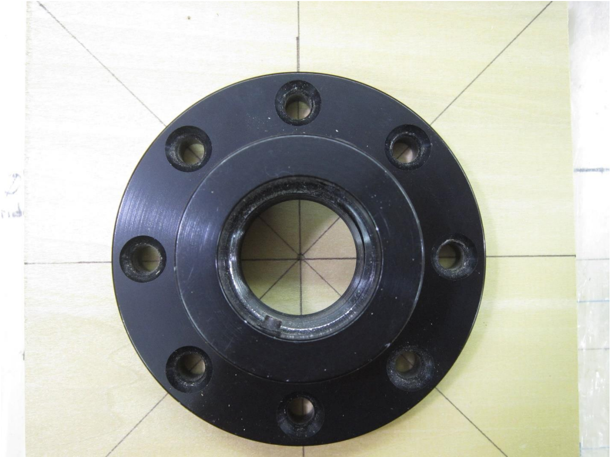
Picture 03 – faceplate on the faceplate board, aligned in the circle so I can mark where the screw holes need to be. You can just see the faceplate board's reference lines through the screw holes in the faceplate. Because of the geometry of my faceplate board, if these lines pass through the center of the faceplate holes, my faceplate is centered on the faceplate board.
