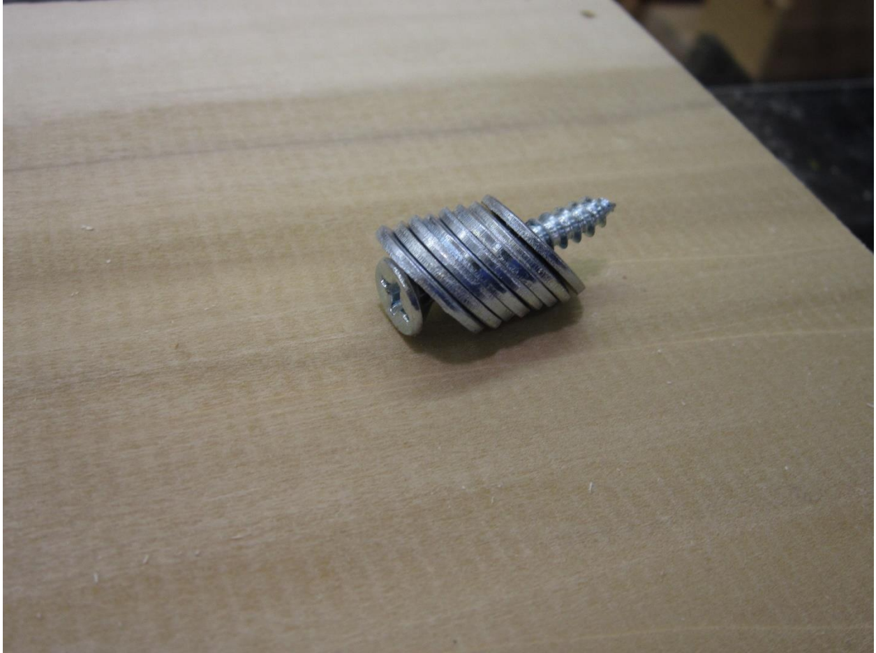
Picture 14 – counterweight made from a wood screw and washers.
